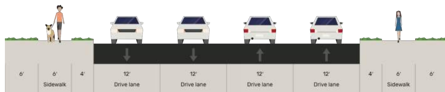
Exhibit 6.5: Major Collector Cross Section
