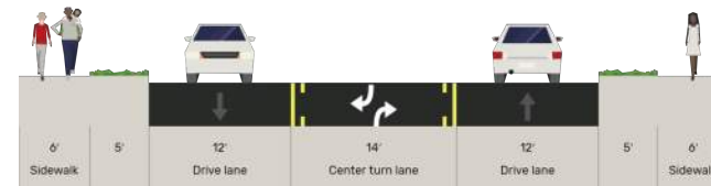
Exhibit 6.6: Minor Collector Cross Section
