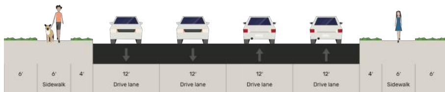
Exhibit 6.5: Major Collector Cross Section
