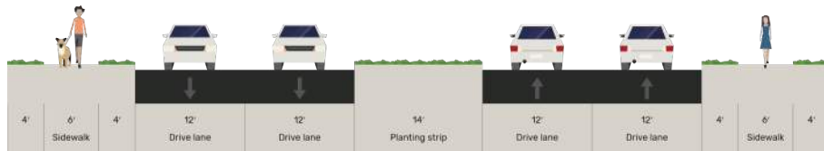
Exhibit 6.4: Minor Arterial Cross Section
