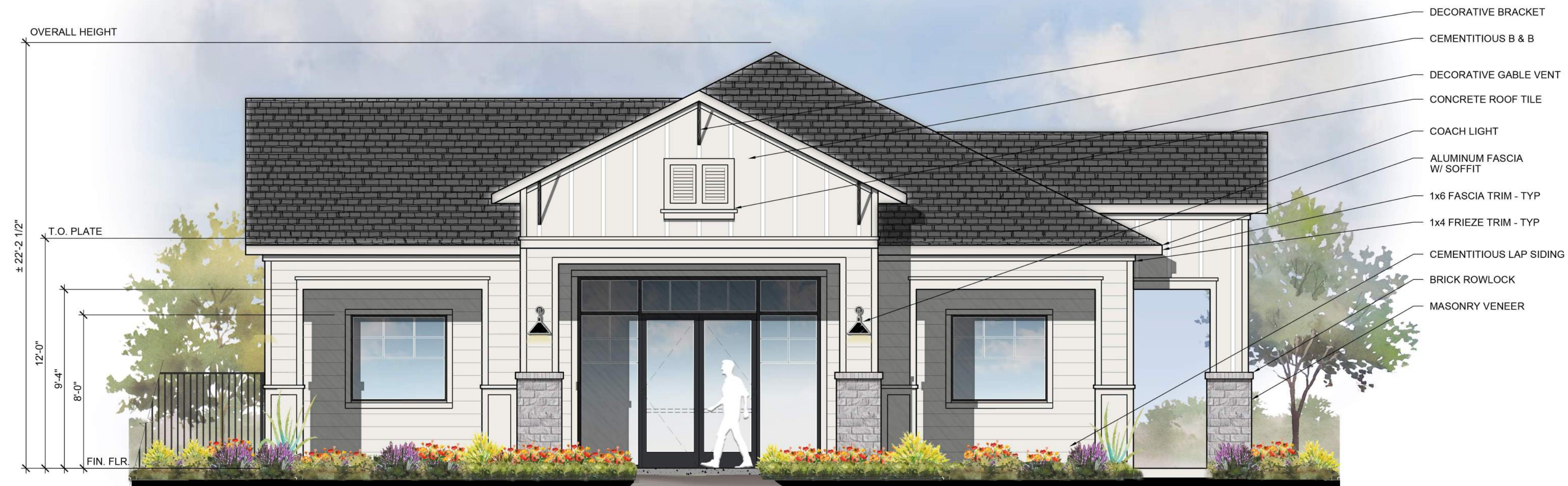
Front Elevation Elevation B - Modern Farmhouse 1/4" = 1'-0"
